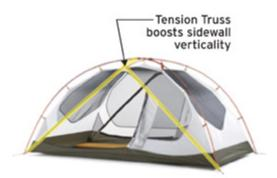
In 2007 REI introduced another space-expanding design feature, the tension truss, on selected tents. A tension truss is a fabric rib attached to a tent seam that, when tent poles are placed in position, makes the seam taut and optimizes the space it provides. It also strengthens a tent's overall architecture, reducing its "wobble" when shaken.
